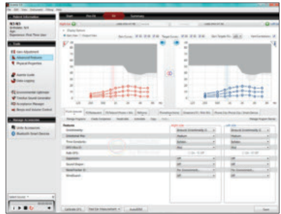
Directional Mix option with temporary visualization of crossover frequency
