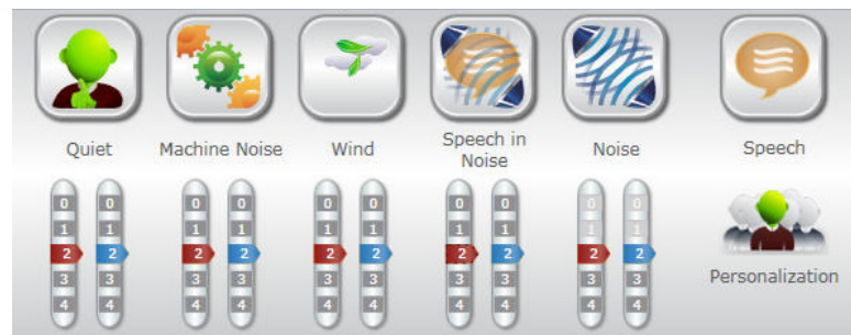
Figure 6. AudioScape icons showing activation of each of the five adaptive algorithms and speech
