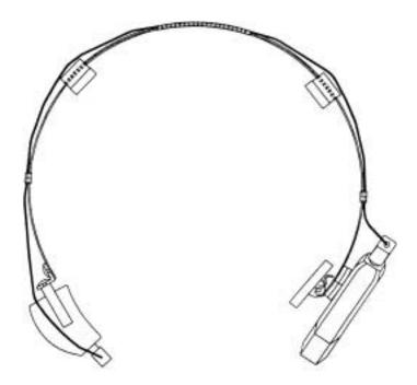
The system consists of a modified power or super power hearing aid, bone oscillator, cord and headband.
