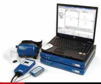
**EcochG:** Electrocochleography is an electrophysiology test that assists in diagnosing cochlear hydrops by comparing the ratio of the summating potential and the action potential.
