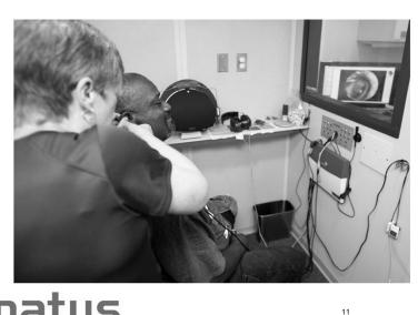
This is the larger of the two booths. Video Otoscopy Astera Audiometer Otoflex Tympanometer Aurical PMM Aurical HIT Box
