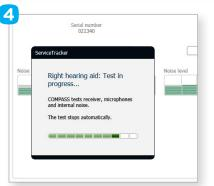
Select the **Start test** button for the hearing device you wish to test. When the test is complete, a dialogue box informs you of the result.
