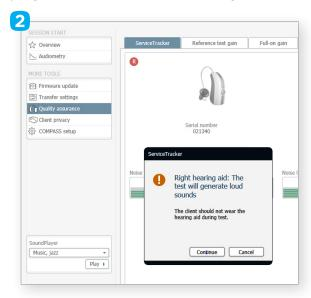
Use the built-in noise level meter to ensure the noise level in the room is not too loud.
