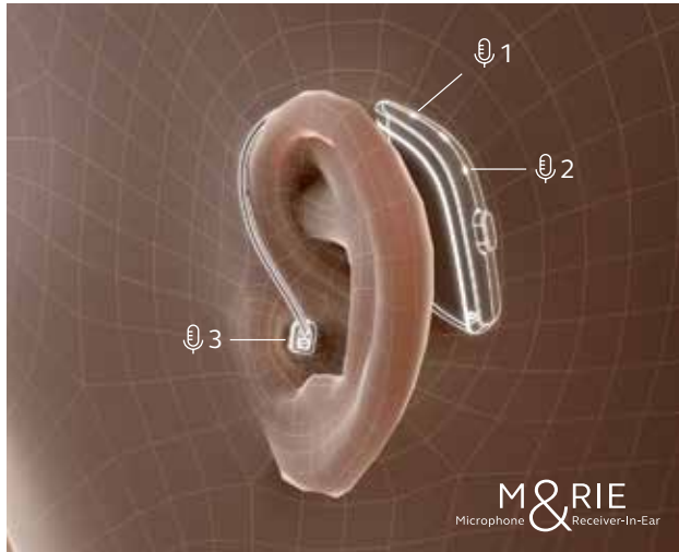
Figure 1. ReSound ONE with M&RIE showing the position of the microphones. The ear canal microphone offers natural protection from wind noise.
