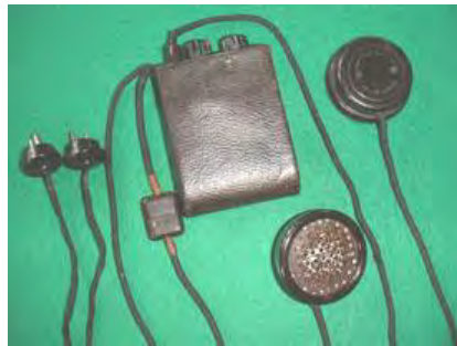
Multitone VPM Vacuum-tube hearing aid
