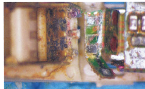
Figure 5: Photo of destroyed metal connections between the battery compartment and internal circuitry.
