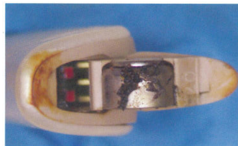
Figure 1: An example of moisture damage
